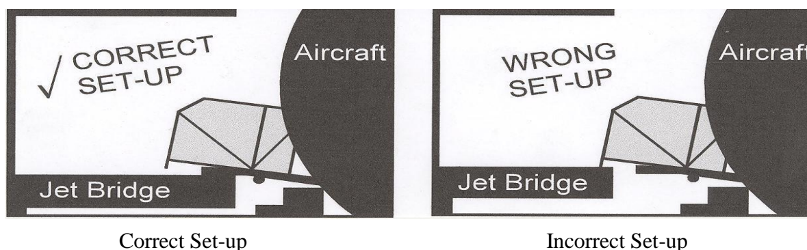
Figure 3 – Side View of Set-up, Air Stair with folding handrails.
