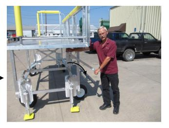
2. Raise or lower the sliding gates by grasping the gate handle to release the latch, slide the gates accordingly.
