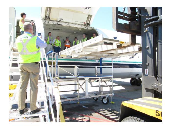
The CWS50-132 737 Combi stand was designed and built for added protection when maneuvering the 737 Combi pallets into and out of the aircraft. The CWS Combi Stand is easily maneuverable and features sliding gates, stabilizer feet and Safegaurd non-skid on walking surfaces and ladder rungs.
