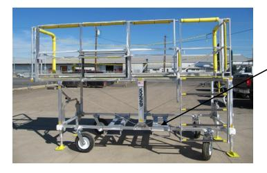
The data plate is located on the frame surface of the Combi Stand.
