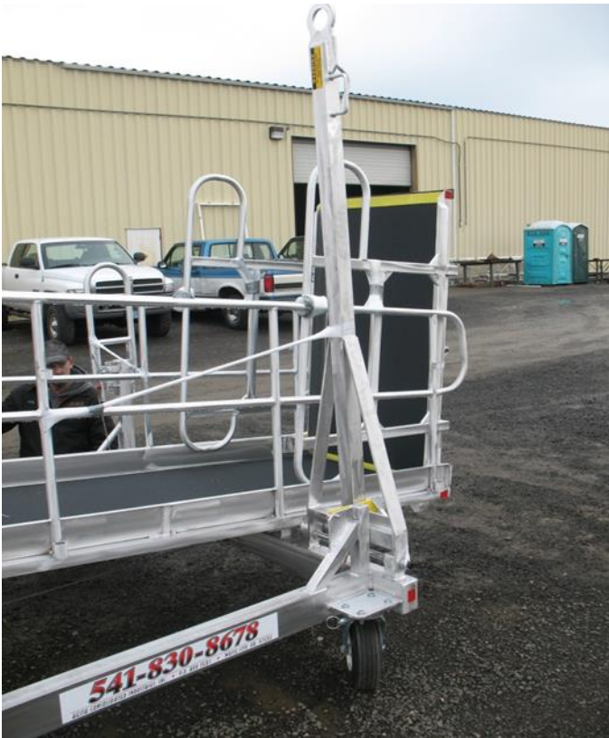
Image showing tow bar raised and latched
