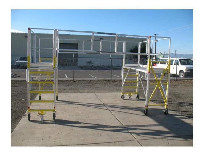
To close the scaffolding, follow the procedure above in reverse order. REMEMBER to make sure that the gates are in the CLOSED LOCKED position when finished with the unit.
