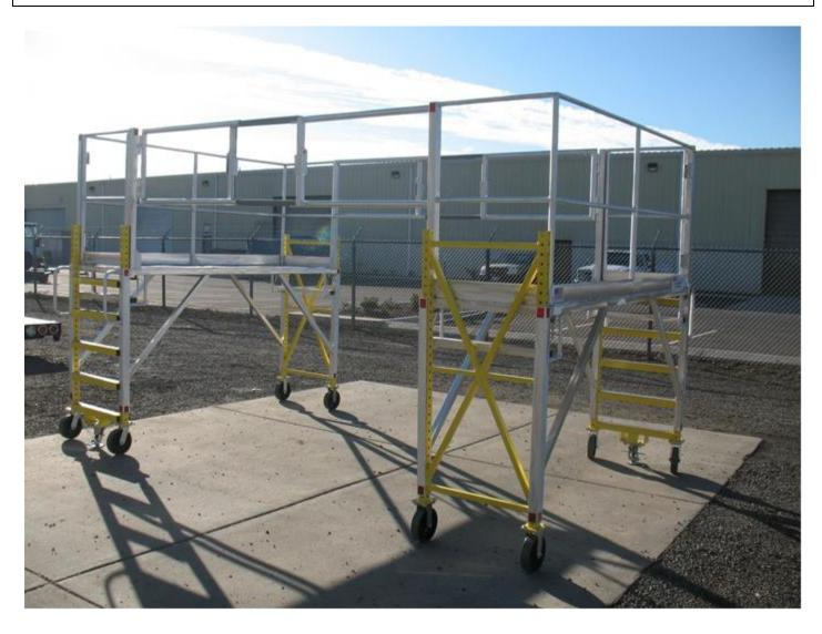
The FS3096 is a multi-purpose scaffolding generally used for ground support equipment maintenance. The scaffolding has the ability to be operated by minimal personnel; one man operation for mechanically lifting or lowering the deck height. Its telescopic gates enable it to be used to work on a variety of equipment. It has a 2000lb weight limit. Polyurethane tread wheels ensure easy maneuvering, but are made to withstand tough terrain if need be.
