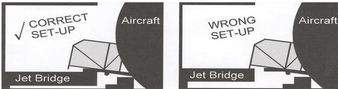
Figure 3 – Side View of Set-up, Air Stair with folding handrails.
