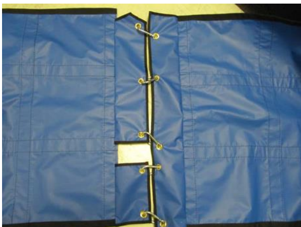
Image showing quick link connection between curtains ↓
