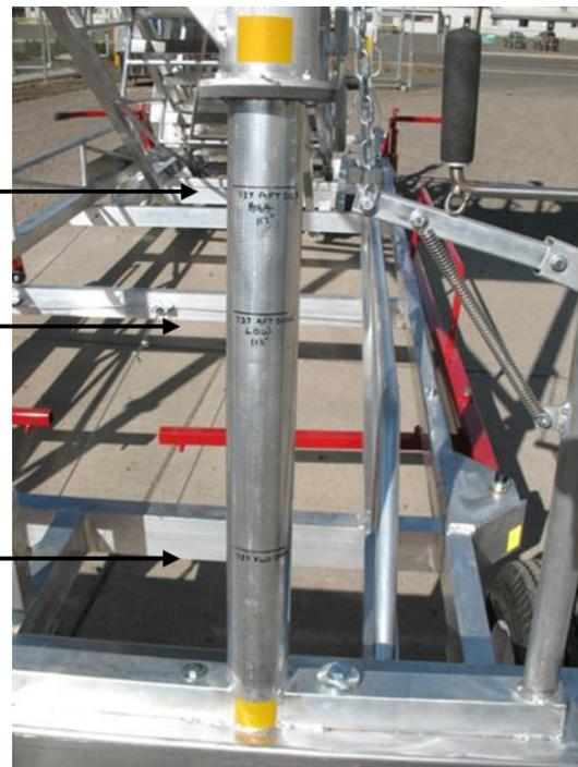
4. The Adjustment Handle has a built in limiting device to prevent the stairs from being raised too far. When the handle comes in contact with the rising bar, it has reached max height, as shown below
