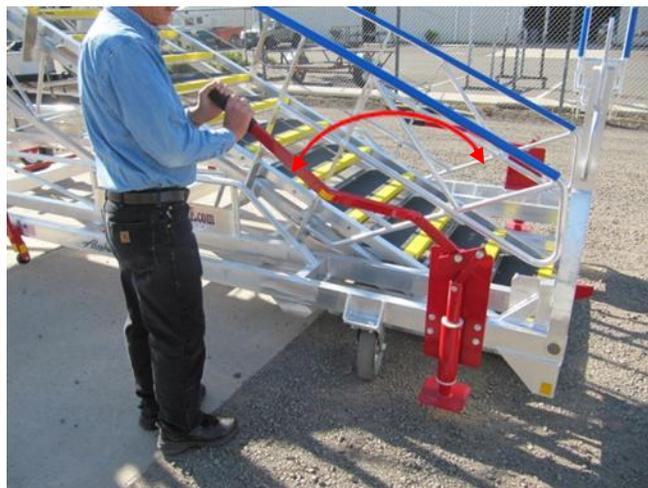
2. The stabilizer will lift the rear swivel wheel off the ground and lock into place once it has been fully engaged.
