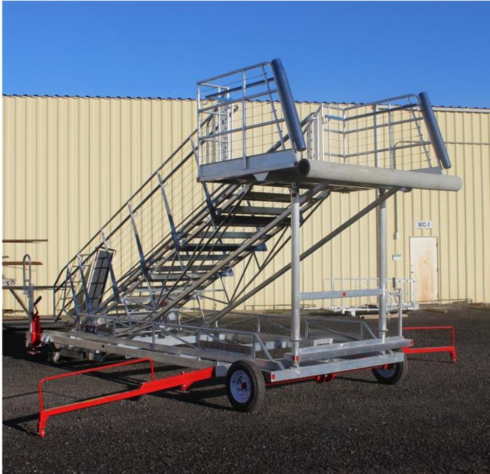
The KCI PXO Fleet Stairs are towable, non-motorized stairs that are easily deployable in less than one minute. The PXO Fleet Stairs feature a hand crank style lifting mechanism for fast and easy height adjustment. The PXO Fleet Stairs also offer outriggers and stabilizer feet as well as cushioning bumpers on the level platform and can be used on the L-1 or L-2 door of the aircraft.
