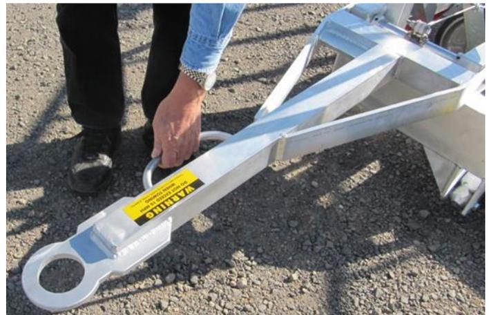
3. Attach the Tow Bar to towing vehicle.
