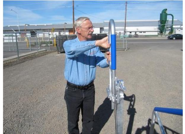
2. While keeping the handle held down, begin pushing the stairs to desired location
