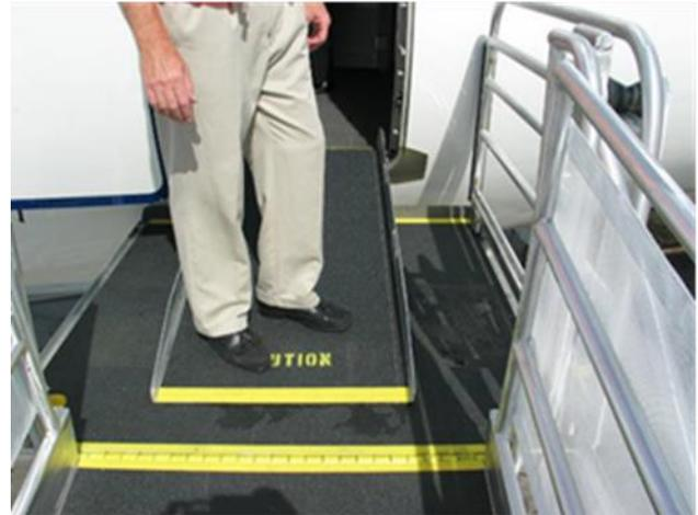
Example of deployed transition plate
