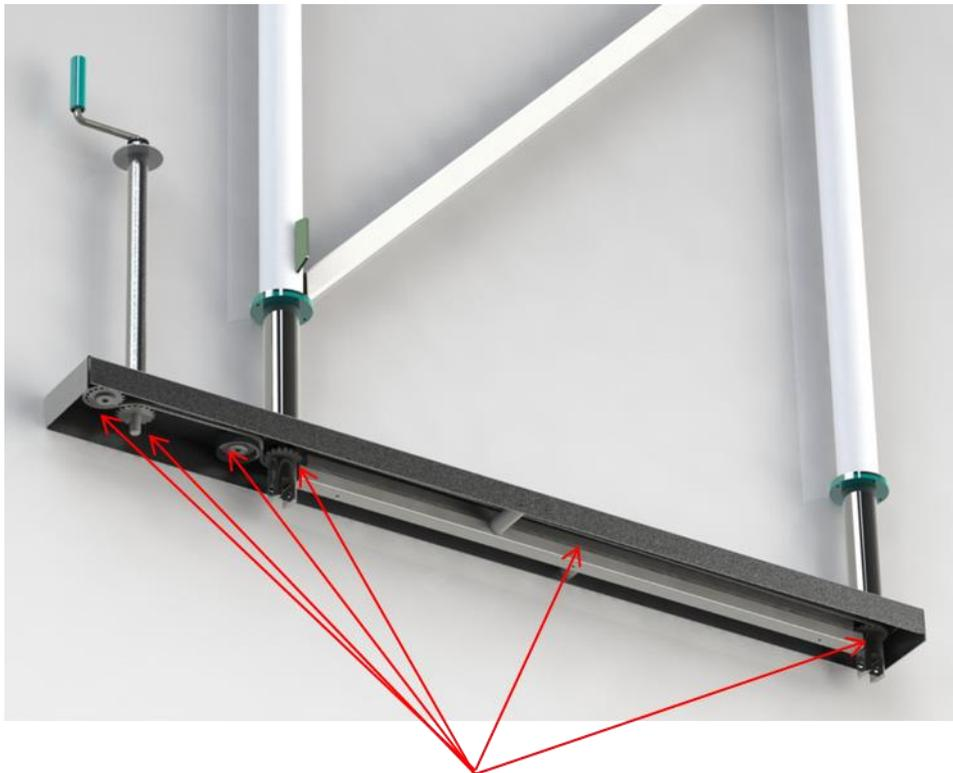
Lifting ram lubrication points
