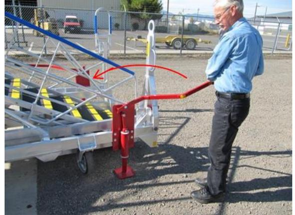
5. The stabilizer will unlock and lower the rear swivel wheel to the ground.
