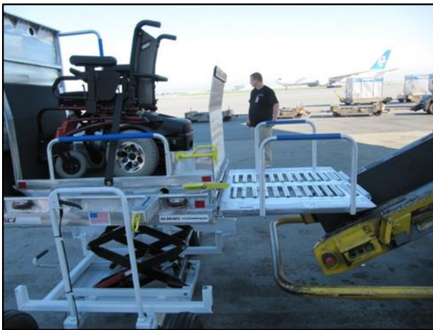
Transition ramp shown level with trailer in preparation to unload
