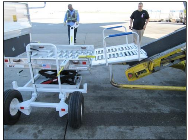
Trailer shown slightly lower than belt loader to receive unloaded barge.
