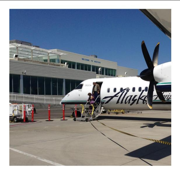
The QS-L1-3306 (Q-Step) is designed to help bridge the gap between the bottom of the aircraft's L1 stairs/handrails and the ground. The design of the Q400 leaves a sizeable gap at ground level and the handrails do not extend out far enough for the last step. The Q-Step addresses these deficiencies, helping to improve safety for the passengers.
